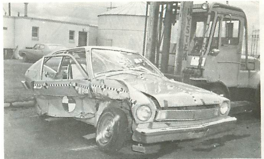
Figure 7-8 TEST NO. 1 – PRE AND POST EXTERIOR VIEWS, CAR NO. 2 - PINTO
