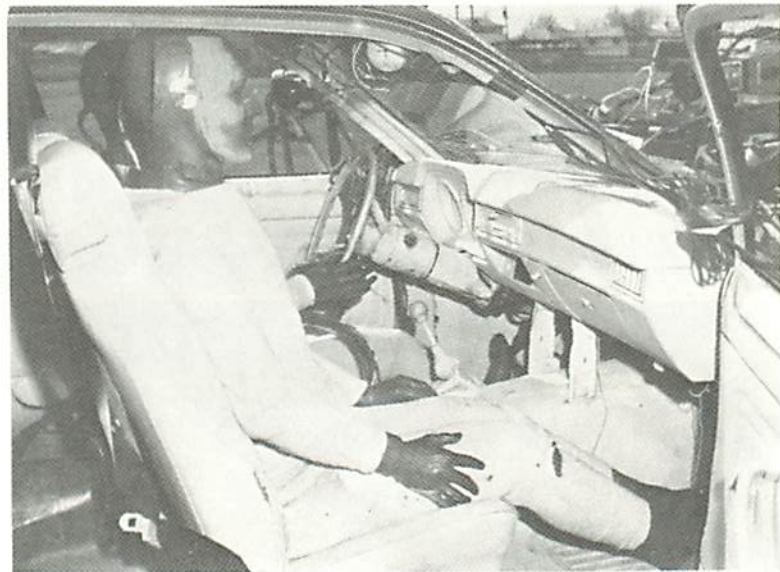
Figure 9-11 TEST NO. 3 – PRE AND POST INTERIOR VIEWS, CAR NO. 2 - PINTO
